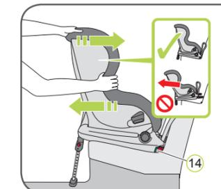
7. Shake the child safety seat to make sure it is safely attached and re-check to the ISOFIX indicators 14 to make sure that both of them are completely green.
