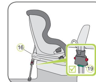
6. Push both adjustment buttons 18 and pull out the support leg 17 until it rests firmly on the floor of the vehicle. The support leg indicator 19 must be completely green.
