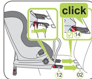
3. Grasp the child seat with both hands and slide the two locking arms 12 firmly into the insert guides 02 until the locking arms engage with a clicking noise on both sides. The green ISOFIX indicators 14 must now be visible on both sides.
